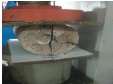
Figure -7 split tensile test
